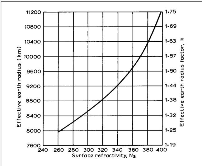
**Fig 12.9: Effective Earth radius corresponding to various values of surface refractivity. A curved ray-path drawn over an Earth section between terminals may be rendered straight by exaggerating the Earth's curvature. An average value often used is equal to 1.33 times the actual radius; this is sometimes referred to as the four-thirds Earth approximation. (Based on CCIR Report 244.)**
