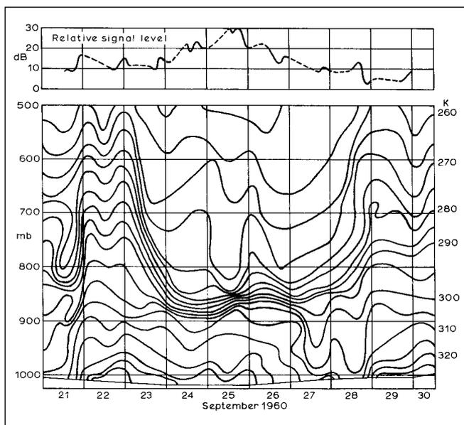
**Fig 12.21: The relationship between variations in potential refractive index in the atmosphere and signal strengths over a long-distance VHF tropospheric path. (With acknowledgements to *J Atmos Terr Phys*, Pergamon Press.)**
