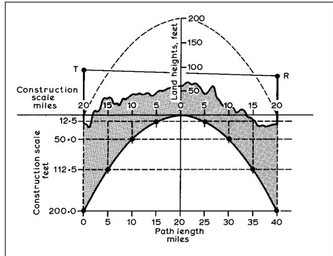
**Fig 12.23: Construction of a 'four-thirds-earth' profile from data in Table 12.9. Land heights are measured upward from the lower curve. On this diagram, rays subjected to 'normal' variations of refractive index with height may be represented by straight lines**
