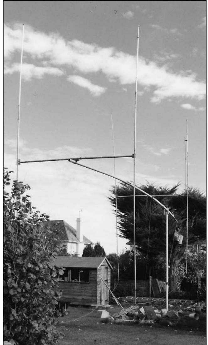
Fig 13.41: 12 metre (40ft) mast and 14MHz quad in the folded over position
