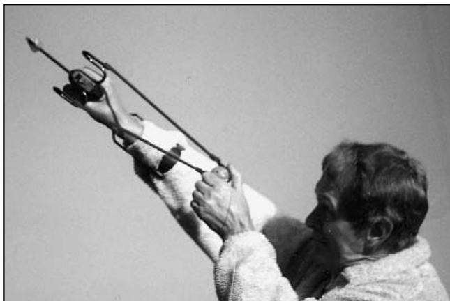
Fig 13.43: An antenna support catapult launch pad. The catapult is held nearly upside down so that the line does not get caught up with anything when fired. It is advisable to gain proficiency with few practice runs in an open space before using it to secure an antenna support.
