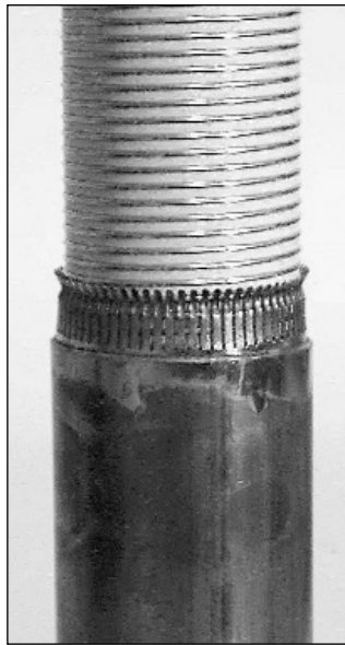
Fig 15.93: W6AAQ's DK3 mobile antenna (not to scale). The control box is located by the driver and power obtained from either the rig supply or the cigar lighter socket. The original had relay switched capacitors, selected from the drivers control box, to match the antenna on the lower frequencies
