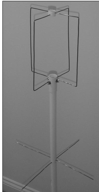
**Fig 16.87: K5OE Eggbeater II without weatherproofing**
