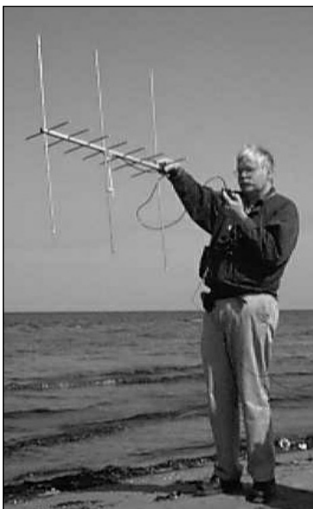
Fig 21.3: Andy Thomas, operating as YL/G0SFJ/P, and working through SO-50 from Riga. He used an Arrow antenna and 5W from a Kenwood THD-7E
