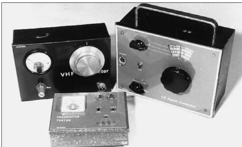
Fig 26.50: Home-made equipment housed in commercial boxes. The items in the foreground and on the right use the paper/Perspex panel system described in the text
