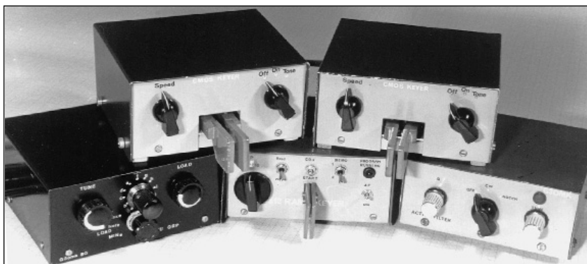
Fig 26.49: Home-made equipment housed in the small cabinet design
