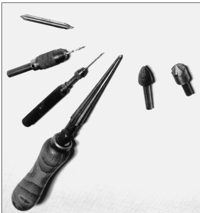
Fig 26.3: Anti-clockwise from the top left: centre drill, pin chuck, pin vice, taper reamer, file burr, countersink
