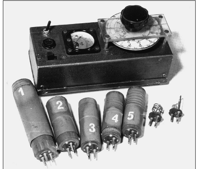
Fig 26.12: Dip oscillator using home-made box described in the text
