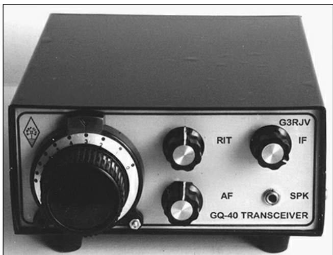
Fig 7.50: GQ-40 exterior view
