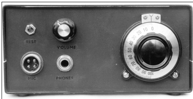
Fig 7.32: Front view of G3TXQ QRP transceiver. On this prototype the TUNE switch is labelled TEST
