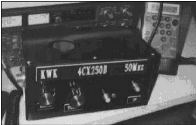
Fig 9.65: The 6m power amplifier
