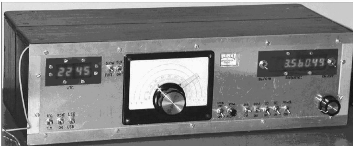
Fig 6.109: Prototype of G0UPL's experimental direct conversion polyphase receiver
