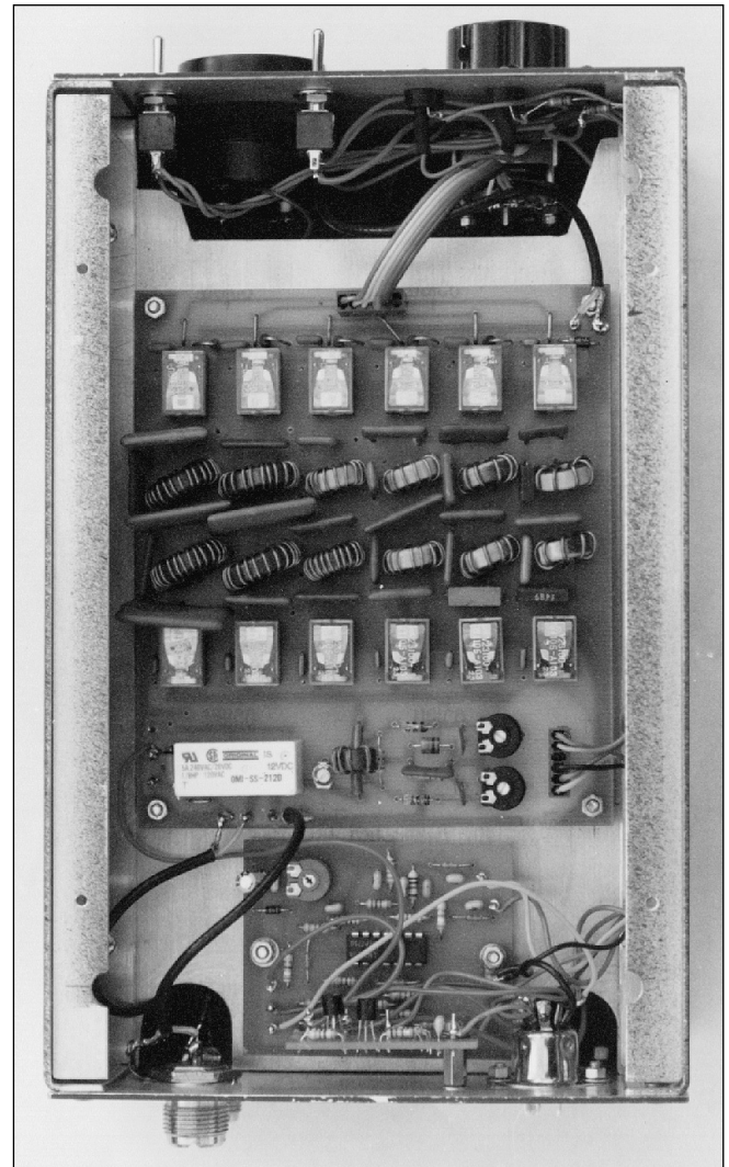
Fig 7.59: Low-pass filter and ALC circuits
