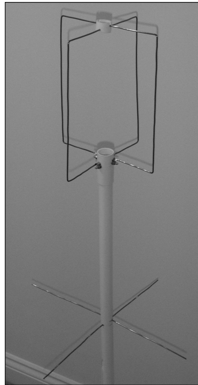
Fig 16.85: Feed point construction detail and phasing line connections for Eggbeater antenna
