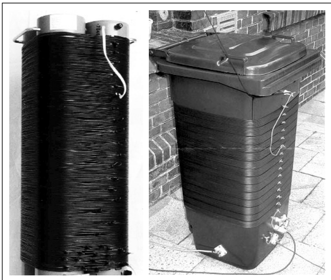
Fig 10.25: Typical Loading coils
