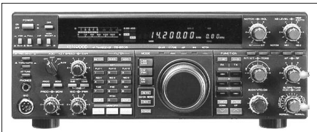
Fig 10.2: The Kenwood TS-850 is the most popular amateur bands transceiver used to receive on 136kHz
