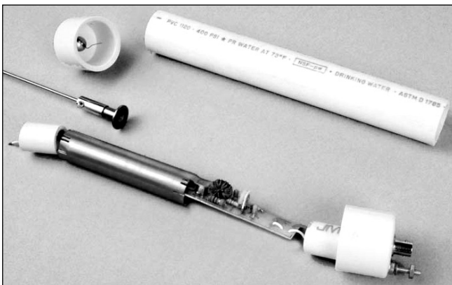
Fig 10.36: The amplifier can be built into the base of the antenna
