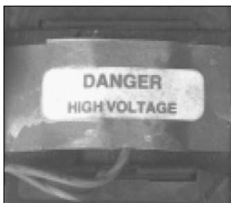
Fig 2.22: Copper foil under the 'Danger' label surrounds the winding and the outer limbs of the core to reduce radiation
