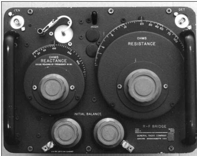
Fig 14.10: General Radio 1606 RF impedance bridge. The indicated reactance value is valid for 1MHz and must be divided by frequency to get the true reactance. Inductive or capacitive reactance is established with the use of the switch located between the two dials
