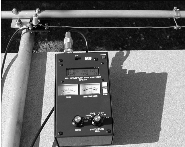
Fig 14.29: Simplified Gamma match by G3LDO, uses hard drawn copper wire as the gamma rod. Connection of the gamma rod to the antenna element is achieved using a hose clamp. A Philips capacitor is used as a reactance correction capacitor, which can be replaced with a fixed mica capacitor of the correct value (see text) once the adjustments are complete.
