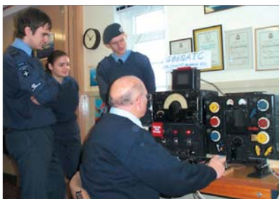
To celebrate the 60th anniversary of the formation of the Air Training Corps, Peter Park, GM3PIP, set up and made several 40m contacts using his WWII-vintage T1154 and R1155 at the headquarters of the Turriff squadron in Aberdeenshire.
