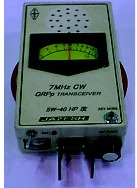
A fine QRP transceiver with built-in keyer and paddles, built by JA2ESR.
