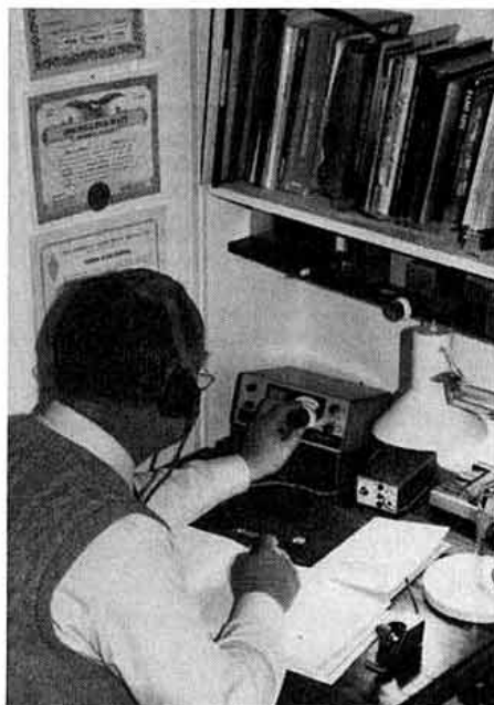
An HF QRP Station need not be large or expensive. Ronnie Marshall, GM4JJG, an active Scottish QRP operator uses an HW8 with a few ancillary items and a simple wire antenna to form a compact complete station.
