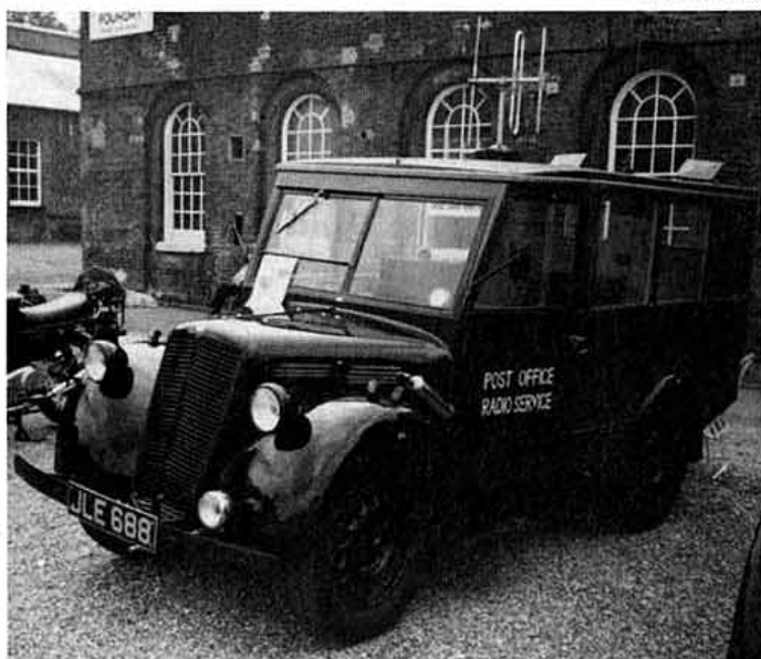
A fibreglass-bodied vehicle used by the Post Office Radio Service, fore-runner of the RIS, seen recently at Chatham Historic Dockyard in Kent. Note the three-element Yagi on the roof.
