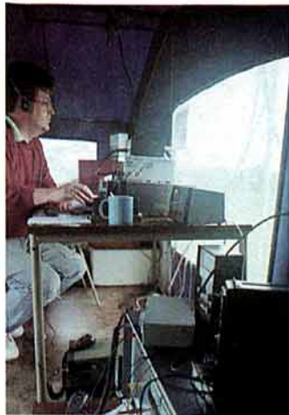
Ian, G4DHA, operating the 1.3GHz station of the Flight Refuelling Amateur Radio Society with the 2.3GHz equipment in the foreground.
