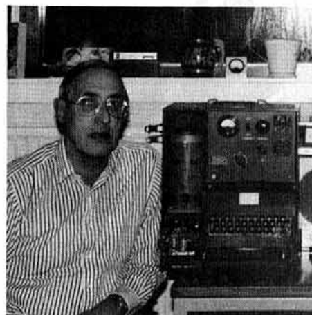
Dick Rollema, PA0SE, with a working 1944 German army 'Feldfernschreiber' machine on loan from PA0AOB.
