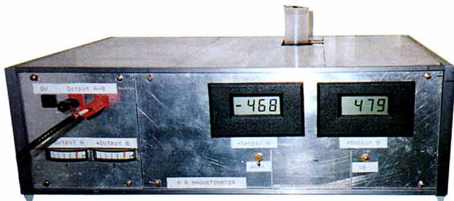
The magnetometer front panel with jam-jar unit protruding through the lid.
