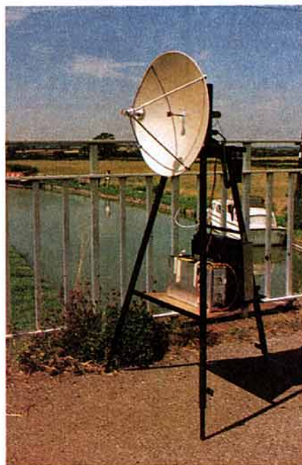
. . . . working G3HBW/P at Stanton Lock, 10.7km distant. Note the Cassegrain dish feed.
