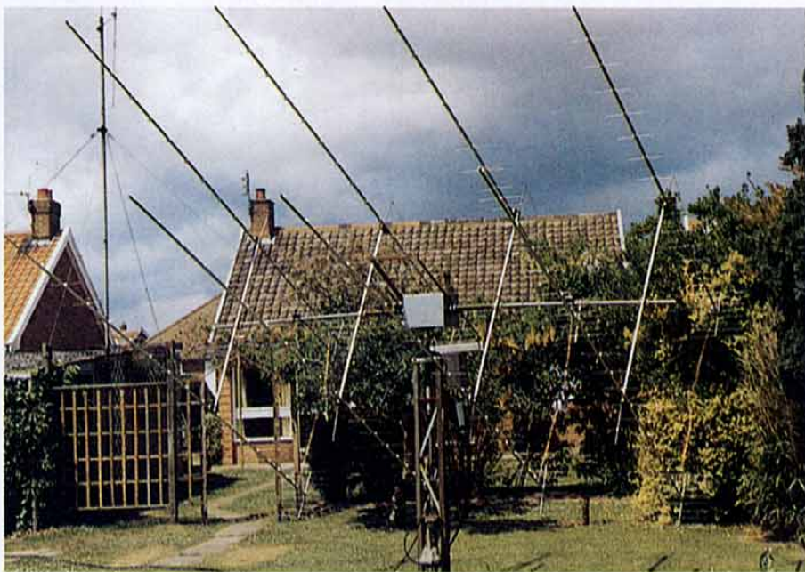
Doug Mallett's, G3HUL, home constructed 430MHz EME antenna system utilises 8x28-ele Yagis.
