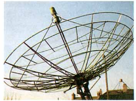
David Jones', GW3XYW, dish is 22 feet (6.7 metres) in diameter. This impressive array provides effective earth-moon-earth (EME) operation on the 23cm (1.3GHz) band.
