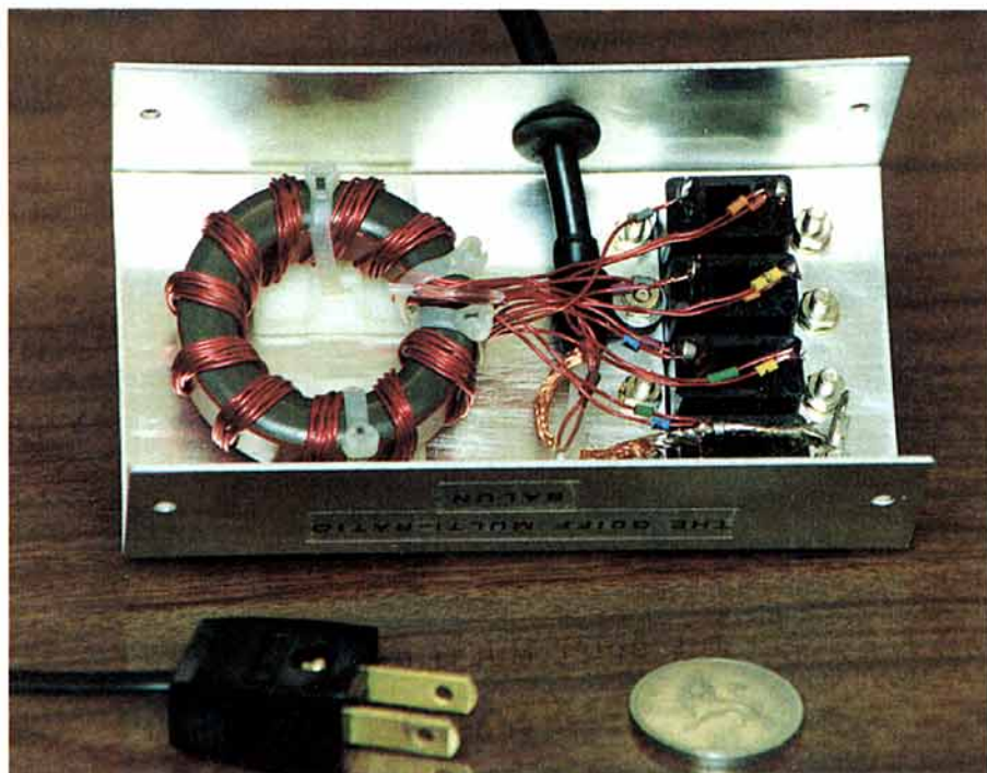
Graham Spinney's HF balun is based around a T200-2 red powdered iron core. Four American chassis mounted mains sockets provide the antenna outputs.
