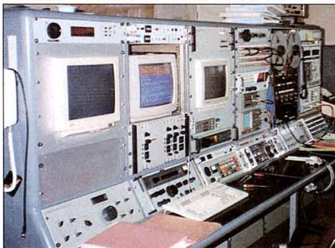
Most types of data transmission can be demodulated and identified on this impressive console which also has long term audio recording facilities.
