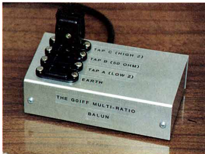
The GOIFF multi-ratio balun provides three taps for efficient antenna matching over a wide bandwidth.
