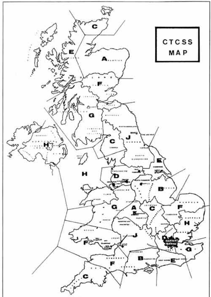
The UK is divided into 23 areas, sharing nine sub-audible tones. Map supplied by the RSGB Repeater Management Group.
