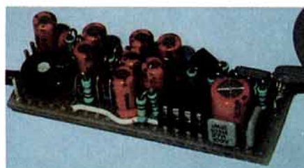
This audio processor was designed by PE1CXO and built on a 2½ x 1" (64 x 25mm) PCB by PA0HUP.
