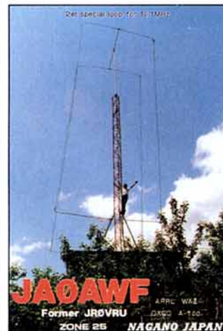
The impressive 2-element loop antenna used by Yoshi, JA0AWF, in Nagano, Japan. He is active on 10.1MHz.
