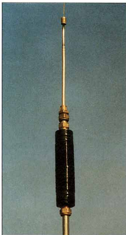
Fig 3: Coil former construction and dimensions will depend on the frequency in use.
