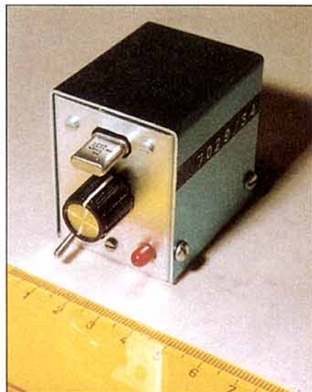
DJ4SB built this ONER transmitter which gives 1.2W on the 40metre band.
