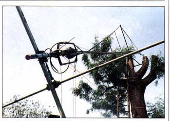
Harry Booth, ZS5AEE (G3BDX) sent in these photographs of this unique antenna support at his hill-top QTH. The tree, which was shaped like this when he moved in, offers both support and a tilt-over action. Sadly, the tree is now redundant as Harry moved to Zimbabwe last year and is now Z26JP.
