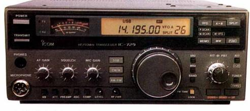
angle. The display indicates frequency to 10 or 100Hz resolution (as selected by the user), mode, memory number and various status indicators for VFOs, scanning and memories.
