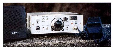
The method of construction used has a number of advantages. Firstly, each module can be constructed and tested separately prior to completion of the transceiver. This should greatly simplify testing and fault finding of the finished product. Secondly, it is possible that the reader may only wish to construct one or two of these modules, perhaps to form part of another unrelated project.
