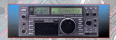
A 50MHz/HF transceiver that allows you to discover the fun that can be had worldwide on the increasingly popular 50MHz band. Features include: 1.8-50MHz, simple all-mode operation, compact size, AF speech compressor, passband tuning, DDS, 105dB dynamic range and band stacking registers. 30kHz-33MHz and 46.2-61.1MHz Rx is possible but not guaranteed.
