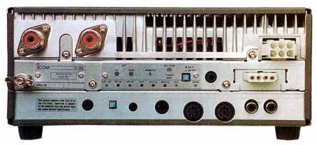
The rear panel carries connections for DC power, key, external speaker and separate antenna sockets for HF and 50MHz.
