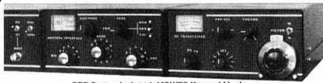
QRP Station built with HOWES Kits and Hardware
