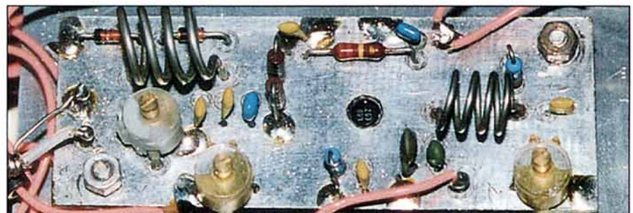
The receive pre-amp uses a 3SK88 Mosfet for low inherent noise.
