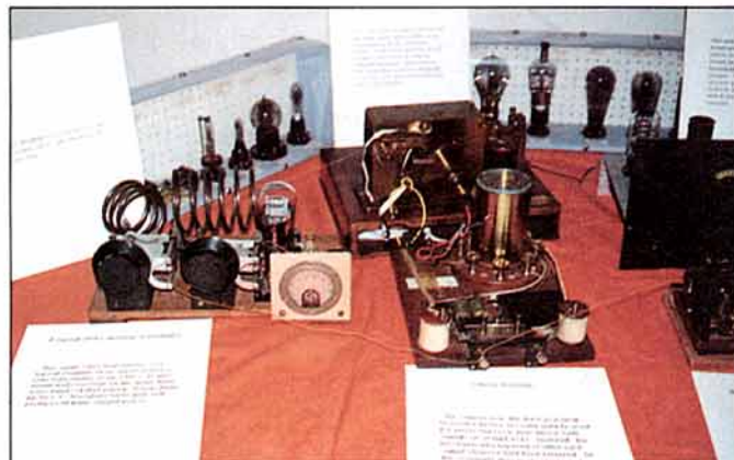
Some of the historic items from the G6NZ collection: Receiving valves pre-1922 (rear left); a very early coherer receiver (front right); and Len Newnham's own 10W transmitter of 30s vintage which gave worldwide coverage on the quiet short-wave bands of that day.
