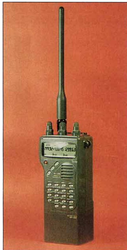
ICOM IC-Δ1E: A versatile three-band hand-held transceiver.
