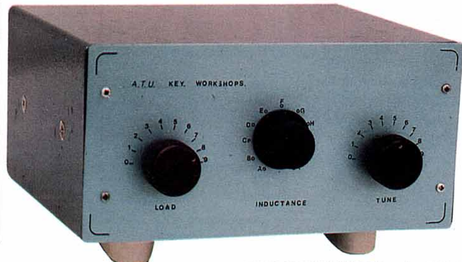
Fig 1: Coil taps select the frequency range.
