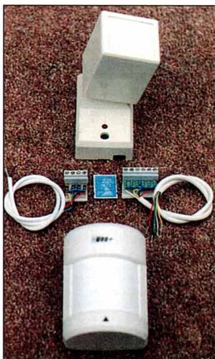
PIR sensors and alarm RFI filters: Top Elkon IR 15 PIR sensor, centre ACT/6030 filters, and bottom ACT/111S PIR sensor.
