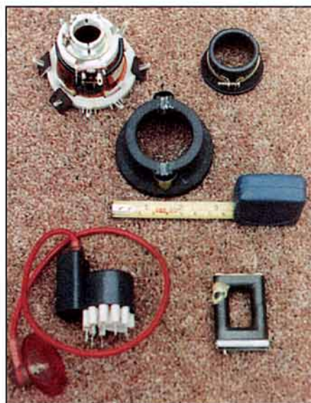
Ferrite components salvaged from scrap TVs. Top left: TV Scan coil assembly. Top right and centre: ferrite deflection yoke cores. Bottom: TV Line output transformer dismantled.
