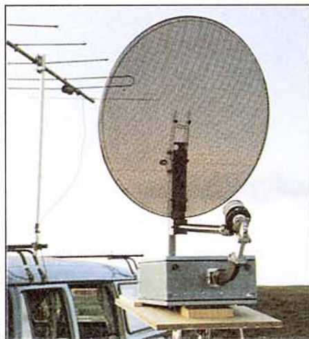
This 60cm satellite dish with an Amstrad horn feed was used by G3PHO/P during the 1993 10GHz Cumulatives. The SSB/CW rig is a modified 'white box' giving 250mW o/p.
