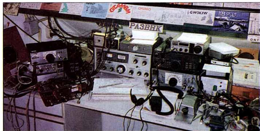
The QRP Station of Robert Van Der Zaal, PA3BHK, a fine mix of commercial and home built equipment: (from left to right) an 80m DSB/CW Transceiver on top of a home built 2m 3W FM Transceiver, a T-Match ATU, the small box on the FRDX500 contains converters for 50, 144 and 432MHz, the large box underneath the TenTec Argonaut II is a home-made 2m AM/FM/DSB/CW 4W transceiver, a transverter from this unit gives 3W on 10m, above the power supply on the right are a 15W linear for 2m and a varactor tripler for the 432MHz band.
