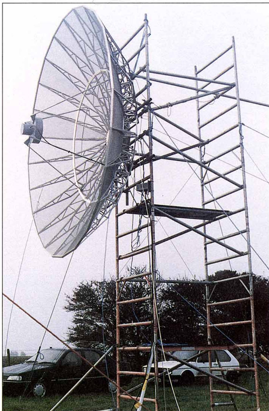
This 4m diameter dish is certain to give the Three Spires Contest Group (G4IEV/P) a good position in the October 1993 1.3GHz Trophy event. The dish knocks down into eight pieces for transporting and can be assembled on site by G4IEV in under two hours. The feed and pivot/steering mechanism is the work of G4HRY.
