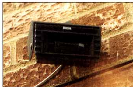
Sensor for Smith's DL05 PIR light switch.
