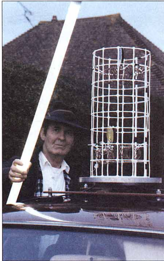
RadCom's Peter Dodd, G3LDO, shows a fluorescent tube being illuminated by RF from a mobile antenna built to G2AJV's design.
