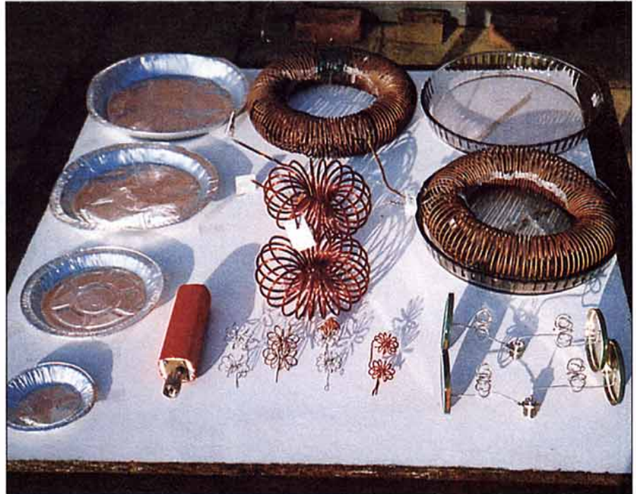
A selection of toroidal antenna components: the cheap aluminium foil picnic plates are very useful for end capacitors. In the centre, coils for 18 and 21MHz can be seen – each must be combined with a twin coil to form a dipole. Rear centre is an 80m coil and to its right a Pyrex dish (more about this next month). The spidery objects are VHF antennas.
