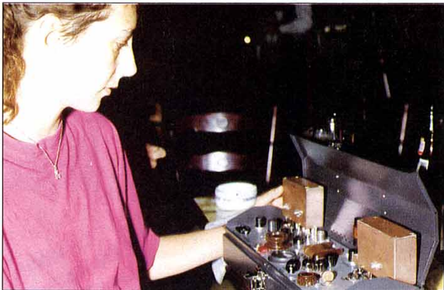
Manuela Groger, DL2MGP, and her own home-made 2 watt QRP transceiver built in a tool box.
