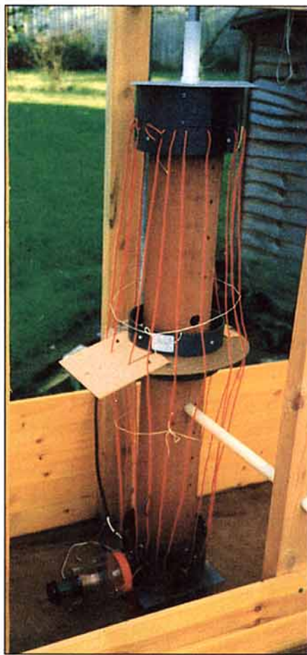
Parallel tuned 18MHz toroidal coil swung into the vertically polarised position. Regular contacts between Kent and the north of Scotland have been made with this antenna at ground level. The vacuum tuning capacitor can be seen inside the clear plastic jar with a red lid at the bottom left of the coil.
