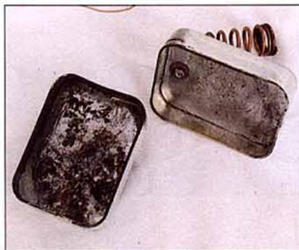
The coil is secured with a nut and bolt through the top of the tin.
