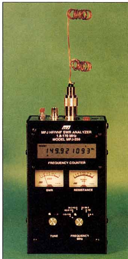
The MFJ-249 being used to check a VHF version of the G2AJV antenna. This instrument is particularly useful for evaluating new designs (or turning ideas into aerials), especially where resonances of early prototypes fall outside the band.
