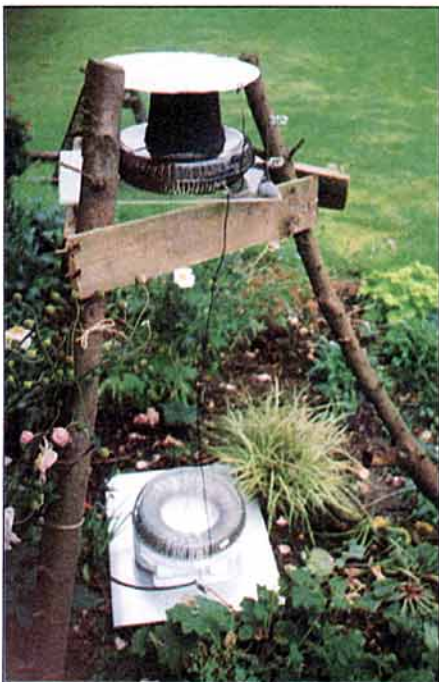
80m double toroid ant using Pyrex dishes to support the coils and aluminium plates as capacity hats.
