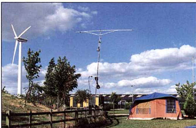
The GB1WAS/GB2WAS aerial farm. On the left is a wind generator used to power the Shelter, with surplus electricity being sold to the national grid.
