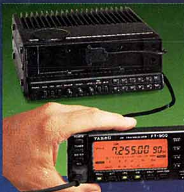
Remote front panel control head measures only 2-1/4" H x 9-1/8" W x 1-1/4" D.
