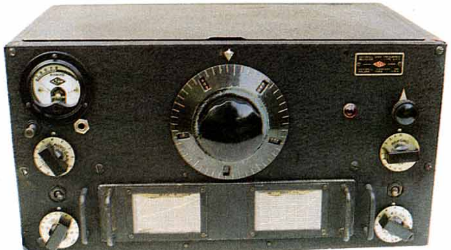
The HRO Senior receiver with bandspread coils and glass valves now in the possession of PA0SE.
