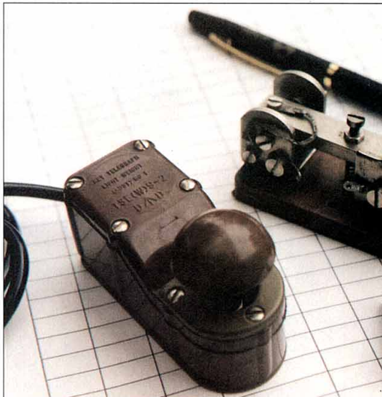
Photo 7: Miniature keys add real fun to portable and/or QRP operations. Shown here are an Australian lifeboat key (L), British lineman/test key (M), and G4ZPY's available-right-now 'Baby' (R). Details in text.
