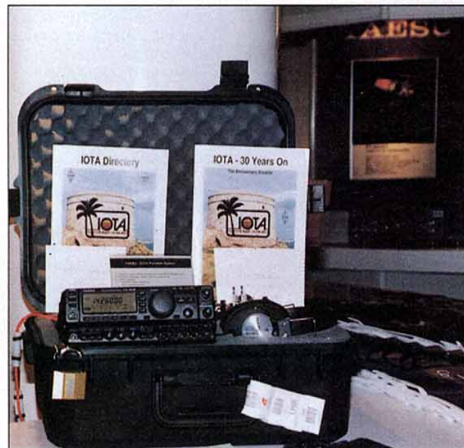
The portable IOTA station, comprising a Yaesu FT-900 transceiver, a lightweight power supply, mic, keyer and wire antenna, all in a splash-proof case.
