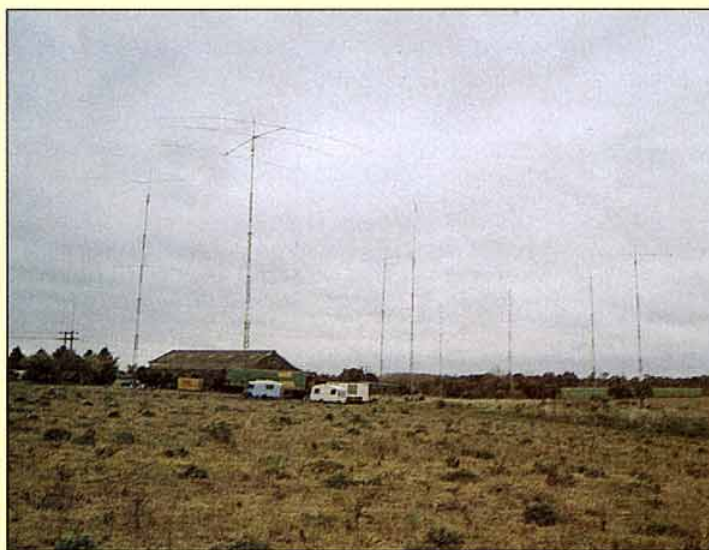
The antennas are (left to right): 15m 5-element beam at 80ft; 10m 5-el at 80ft; 20m 5-el at 100ft; 40m 2-el at 80ft; 10m 5-over-5 with top at 90ft, bottom at 65ft; 15m 5-over-5 with top at 100ft, bottom at 60ft; 40m 3-el at 90ft; 20m 4-over-4 with top at 100ft, bottom at 60ft; 150ft vertical for 160m in the distance. Not shown in the picture is a 160m inverted-vee at 110ft away to the left, and an 80m 4-square (four 63ft verticals) to the right.
