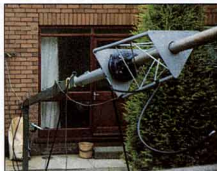
The Tennamast rotator cage for pipe masts.
