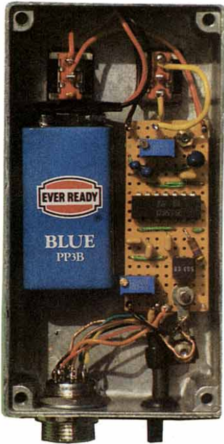
The components are mounted on stripboard.
