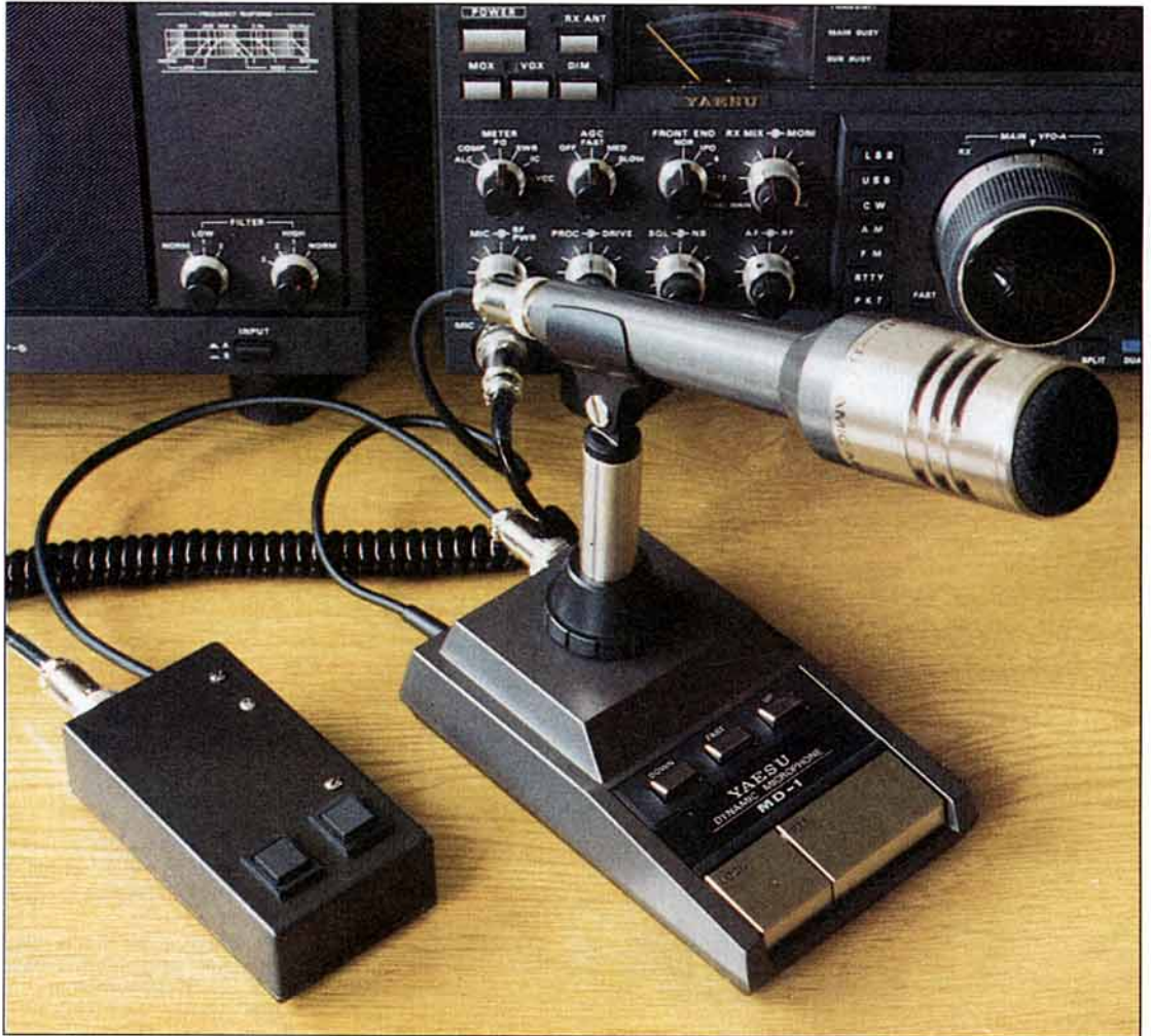
The tuning pulser provides an instant means of causing a transceiver to provide a modulated SSB signal so that aerial or linear amplifier tuning can be done quickly.
