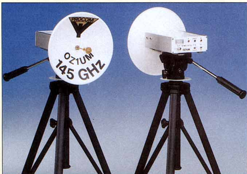
The two 145GHz transceivers consisted of DB6NT's 12GHz injection chain and doubler/amplifier, a double-balanced harmonic mixer with four diodes manufactured in the Russian Salut plants. The aerials are 25cm PROCOM dishes with a backfire feed system.
