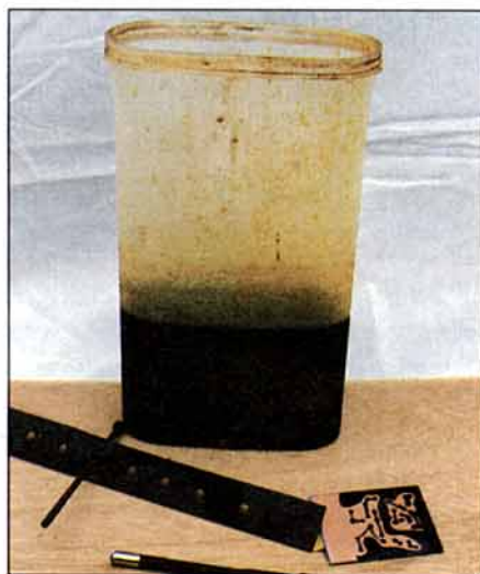
Equipment required to etch PCBs.
