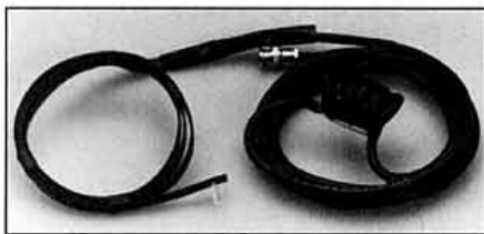
VE2CV's two-metre Ribbon-J antenna showing the current balun formed by coiling a small length of the coaxial feedline.
