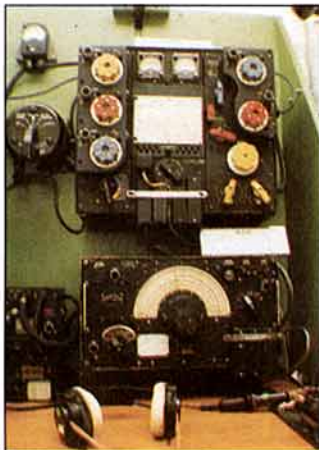
A working T1154/R1155 station in the GB2IWM shack.
