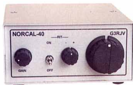
NorCal-40, a 40 metre Super Transceiver kit.
