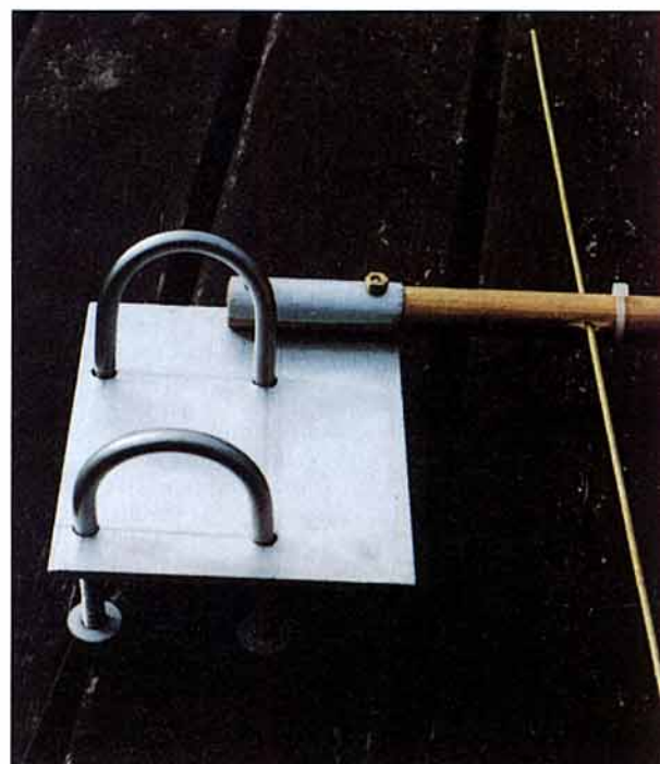
A cheap mast clamp can be made from two U-bolts and some scrap aluminium.
