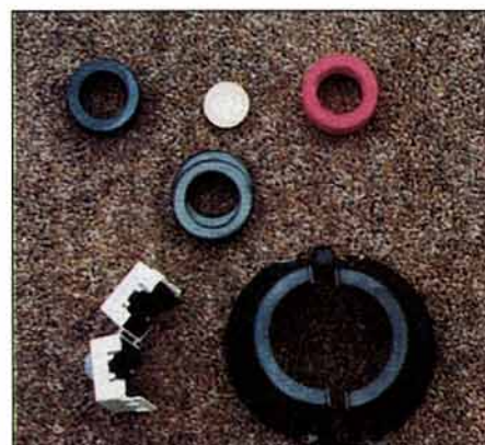
Ferrite rings and cores for EMC use. Top left, Fair-Rite 2643802702. Top right, Philips 4330-030-3445. Centre, a pair of Neosid 28-041-28. Lower left, Maplin BZ34M. Lower right, large CRT deflection yoke ring.
