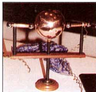
Replica of spherical transmitter used in Sir Oliver Lodge's 1894 demonstration of wireless telegraphy.
