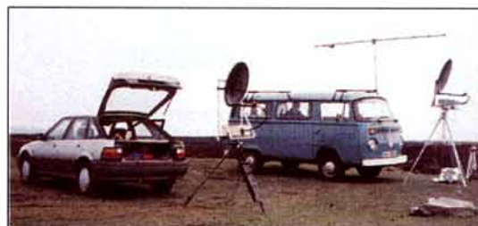
G4EQD/P and G3PHO/P on Houndkirk Moor near Sheffield. Both stations run 250mW to 60cm dishes. The 144MHz beam is used for talkback.
