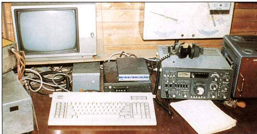
The operating position at RK9CWW BBS in Ekaterinburg. Left to right: AT286 in home made case, Yaesu YVM-1 monitor, 2 x 12V power supply, PK88, home made synthesised VFO, Yaesu FT-902DM and a home made linear.
