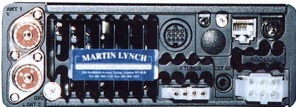
Rear view of IC-706 showing the dual antenna sockets and many other connections.
