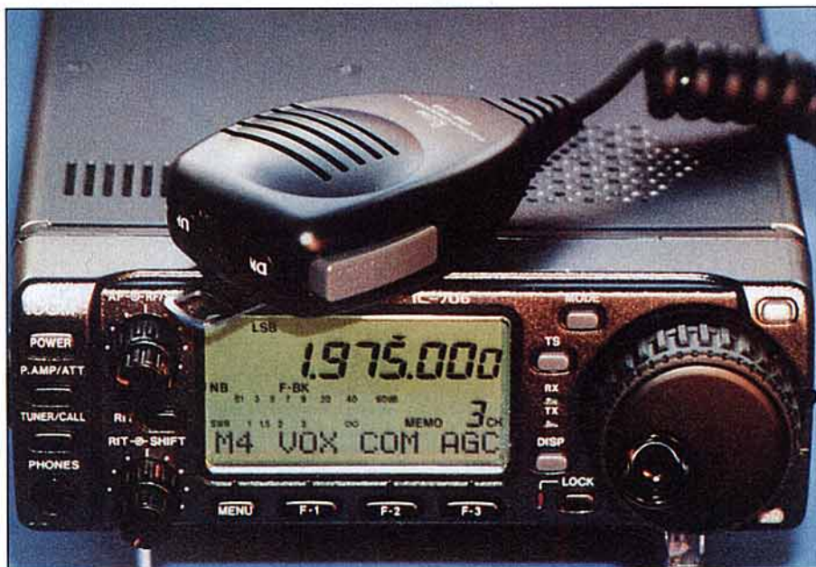
The Icom IC-706 is the smallest 100W HF/VHF transceiver presently available.
