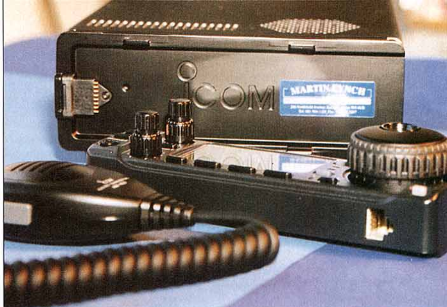
The front panel is easily removed to allow for easy installation in even the tightest spaces.
