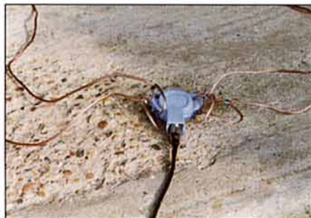
The feedpoint of the MyDEL Multi-Trap dipole antenna.
