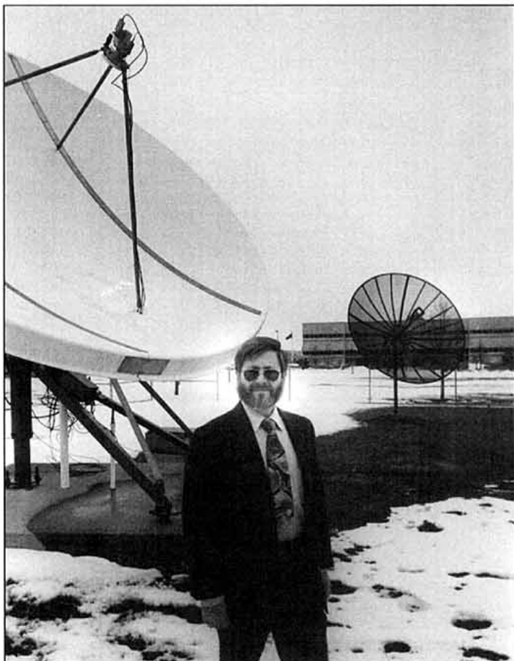
Fig 3: The author standing before the 5-metre (left) and 3-metre (right) satellite TV dishes. Both antennas have been refitted for amateur SETI. Five thousand such systems around the world can provide real-time all-sky coverage.
