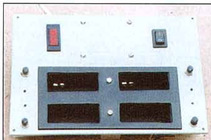
Battery discharger/charger, front panel.
