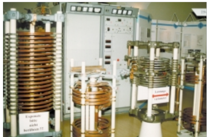
Behind a display of power variometers, a 20kW transmitter made by Funkwerk Köpenick of the DDR.
