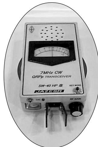
A 7MHz QRP CW transceiver, with built-in keyer, by JA2ESR.
