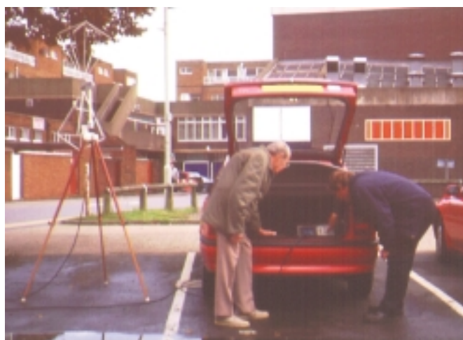
Two radio amateurs measuring spurious emissions in the 144 - 146MHz band from a taxi company's faulty transmitter somewhere in the UK.
