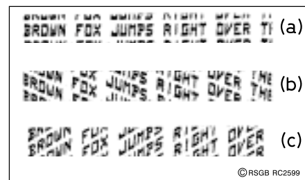
Fig 3: Appearance of Hellschreiber transmissions on a mechanical machine. (a) Transmitter and receiver running at approximately the same speed. (b) Receiver running slow. (c) Receiver running fast. (Source: G5XB's 1981 article)
