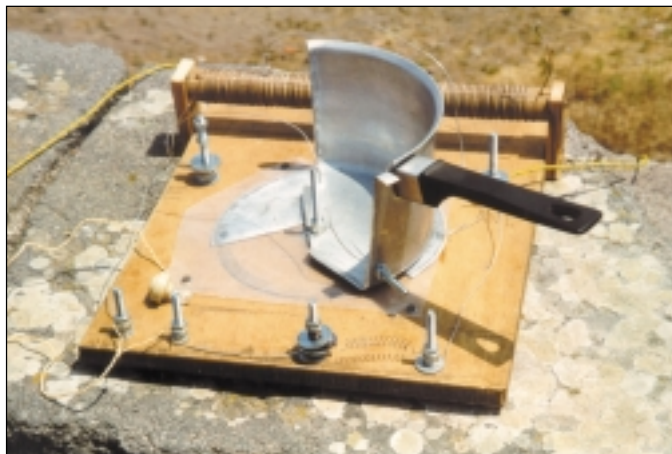
The saucepan-tuned short-wave crystal set.
