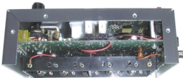
Behind the battery holder, the PCBs.
