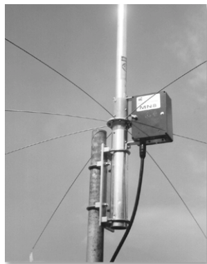
Feed point and radials of the assembled antenna.
