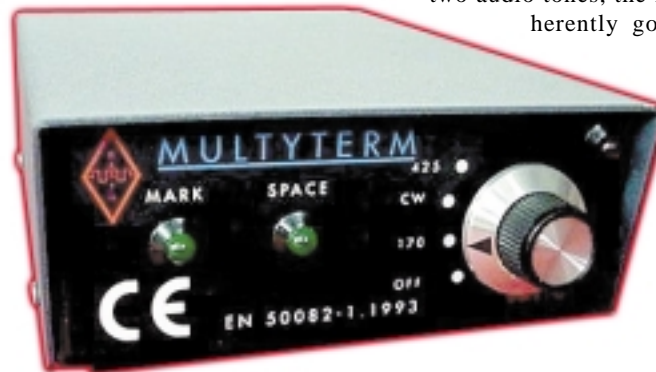
The Multyterm Terminal Unit, available from BARTG as one of its range of products for amateur datacomms. It is designed for use in conjunction with an IBM-compatible computer running the Grosvenor Software Multy suite of programs for PACTOR, AMTOR, RTTY, CW, FAX and SSTV.
