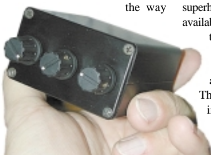
The NorCal SMK-1 surface-mount kit transceiver.
