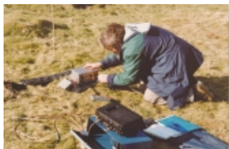
G3PAI injects a known earth current. Down below, G8DSU reads signal strengths from a circle of electrodes.
