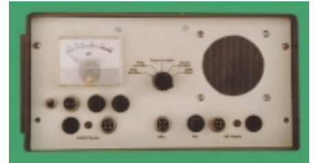
A talk-through box, used to interface the cave radio with an amateur HF or VHF transceiver.
