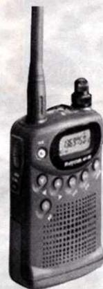
Palm sized dedicated airband scanning receiver. Covers airband 108-136.975MHz VHF 136-180MHz with 99 memories (AM/FM).
