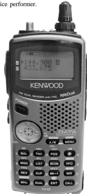
usual memory to VFO transfer facilities. All models except the Kenwood provide a single quick access home channel per band, but only the Yaesu allows the memory structure to be split into groups.
