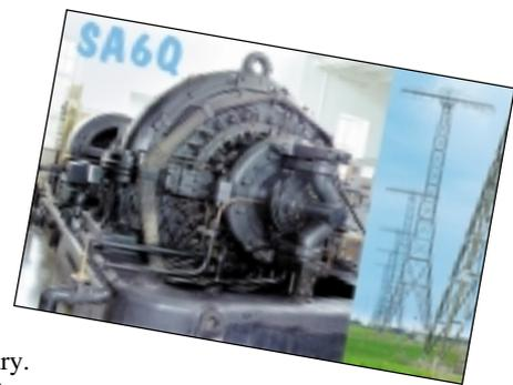
The QSL card sent out to those who worked the 40m station SA6Q. It shows the alternator and the six 127m towers which support the VLF antenna.
