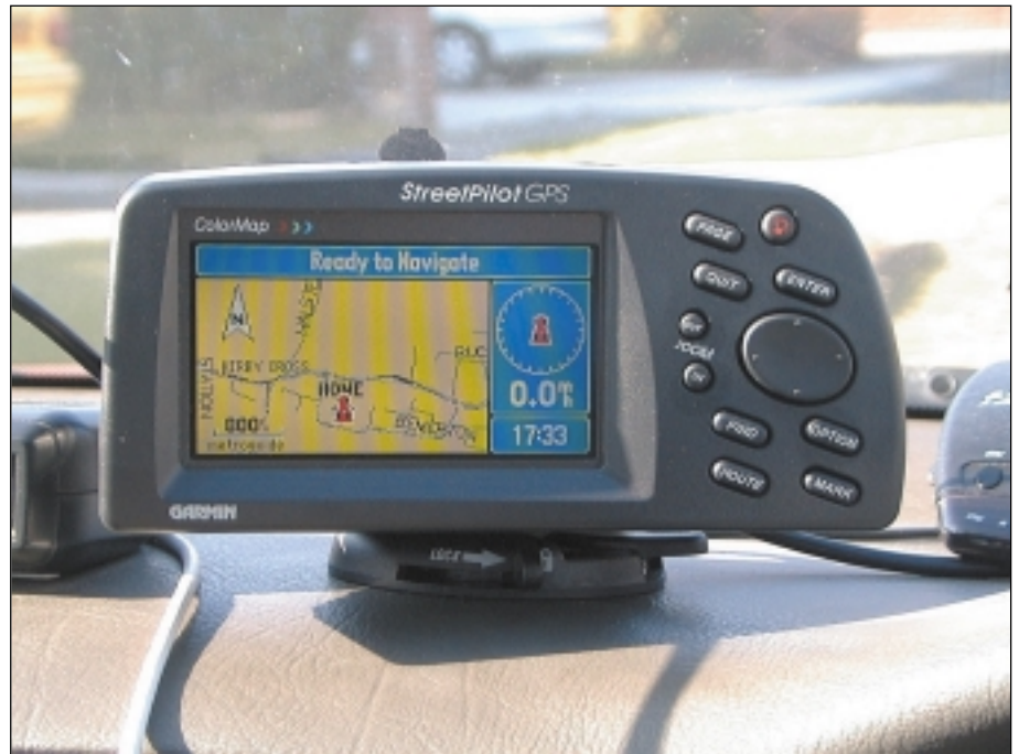
The Garmin Street Pilot - typical of the range of systems available with NMEA output (see text). (G6NHU)
