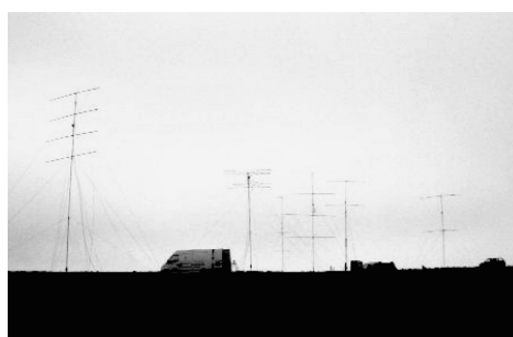
The Northern Lights Contest Group's impressive antennas. From left: 70cm 4x28, 4x21; 144MHz 4x9, 4x15; 50MHz 2x7 on trailer tower; 2x7 on scaffold mast.
